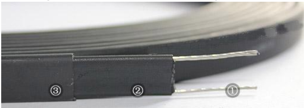
1. Wire core; 2. Conductive plastic layer: flame-retardant PTC; 3. Insulation layer: flame-retardant polyolefin
